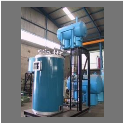
Thermopack Oil Boiler
