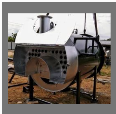
Oil Fired Steam Boiler
