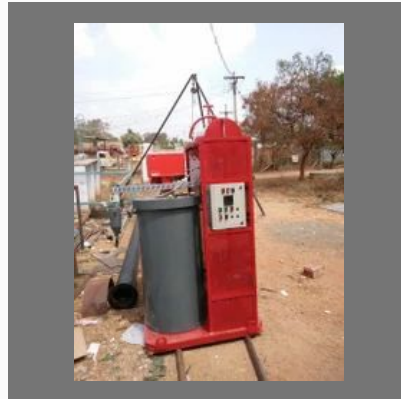
Packaged Steam Boiler
