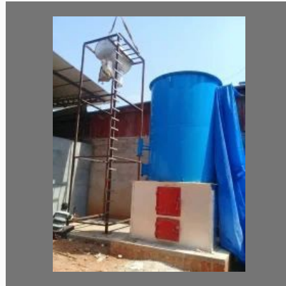
Wood Fired Thermic Fluid Heater
